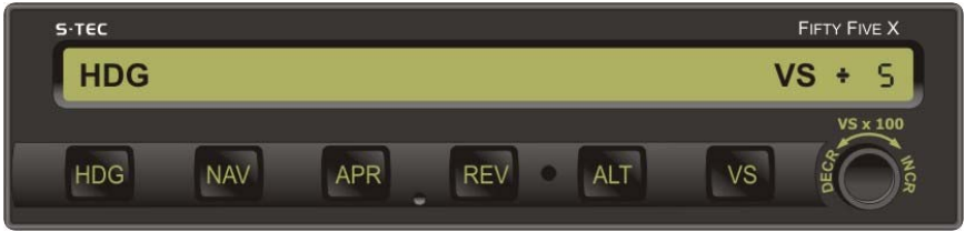
Fig. 3-12. AP Display, HDG and VS Modes Engaged
