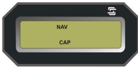
Fig. 3-3. Remote Annunciator Display, NAV Mode Engaged, CAP Condition
