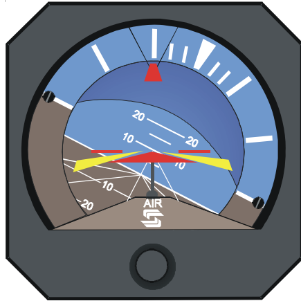
Fig. 3-39. FD Display, FD/AP Mode Engaged
