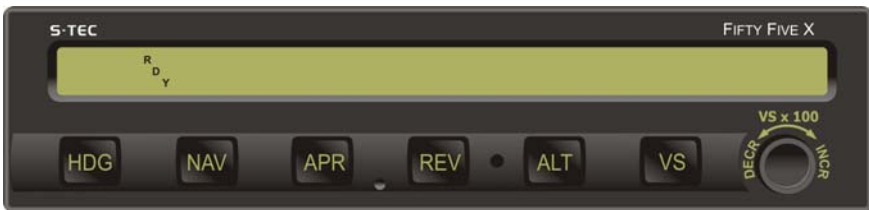
Fig. 2-3. AP Display, Ready for Operation
