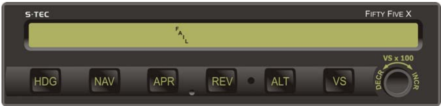
Fig. 2-4. AP Display, Programmer/Computer Failure
