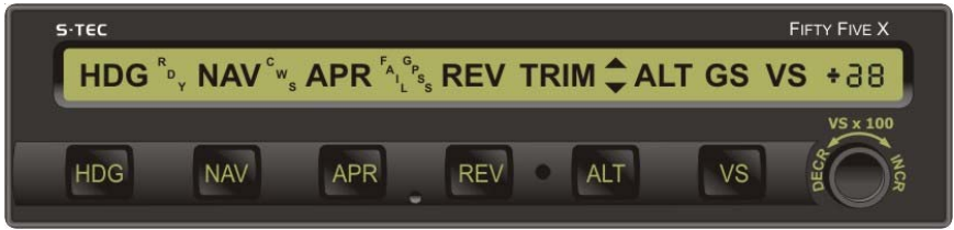
Fig. 2-1. AP Display, All Annunciations at Power-Up
