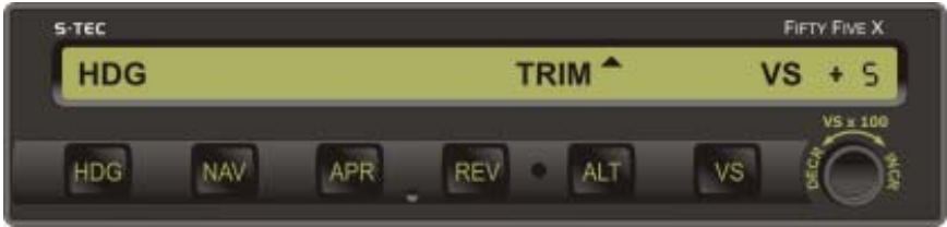
a. TRIM UP in Progress
