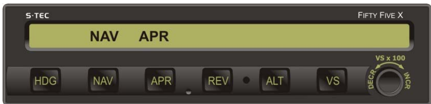
Fig. 3-24. AP Display, NAV APR Mode Engaged, Track LOC Back Course Outbound
