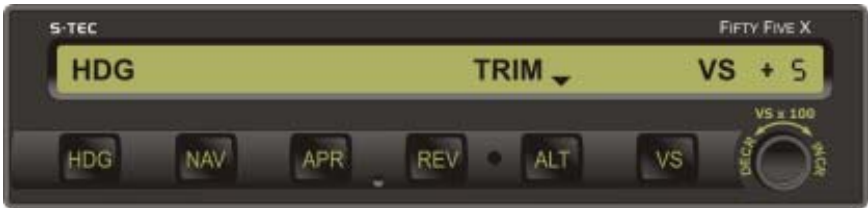
b. TRIM DN in Progress
