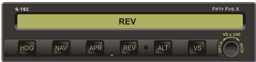
Fig. 3-34. AP Display, REV Mode Engaged, Track VOR Front Course Outbound
