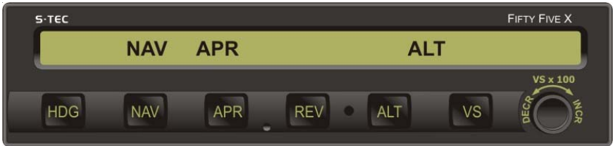
Fig. 3-17. AP Display, NAV APR and ALT HOLD Modes Engaged
