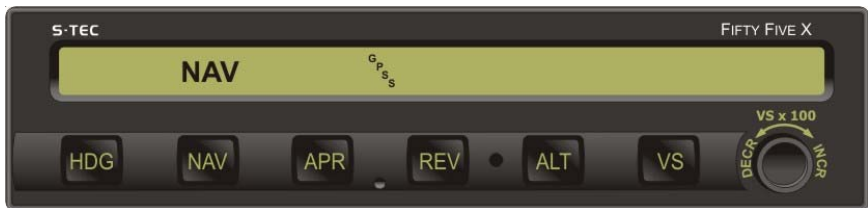
Fig. 3-9. AP Display, NAV GPSS Mode Engaged
