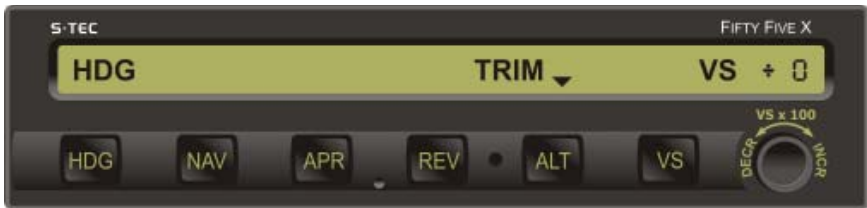
b. HDG and VS Modes Engaged, 0 FPM, TRIM DN Required
