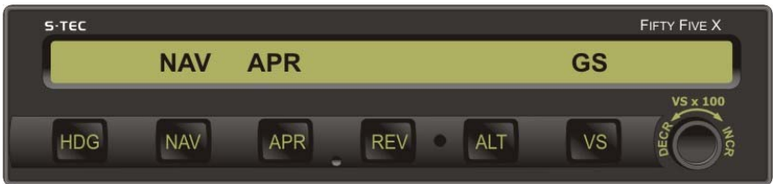
Fig. 3-19. AP Display, NAV APR and GS Modes Engaged
