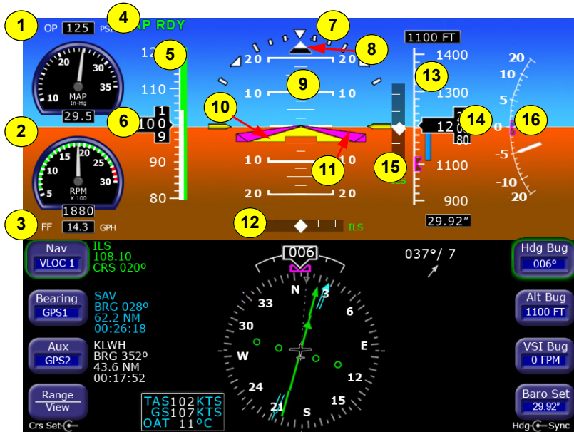
Figure 2. EXP5000 Upper Half Display Symbols
