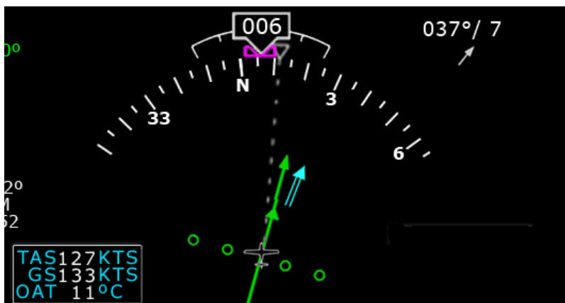
Figure 4. EHSI Arc (120°) View
